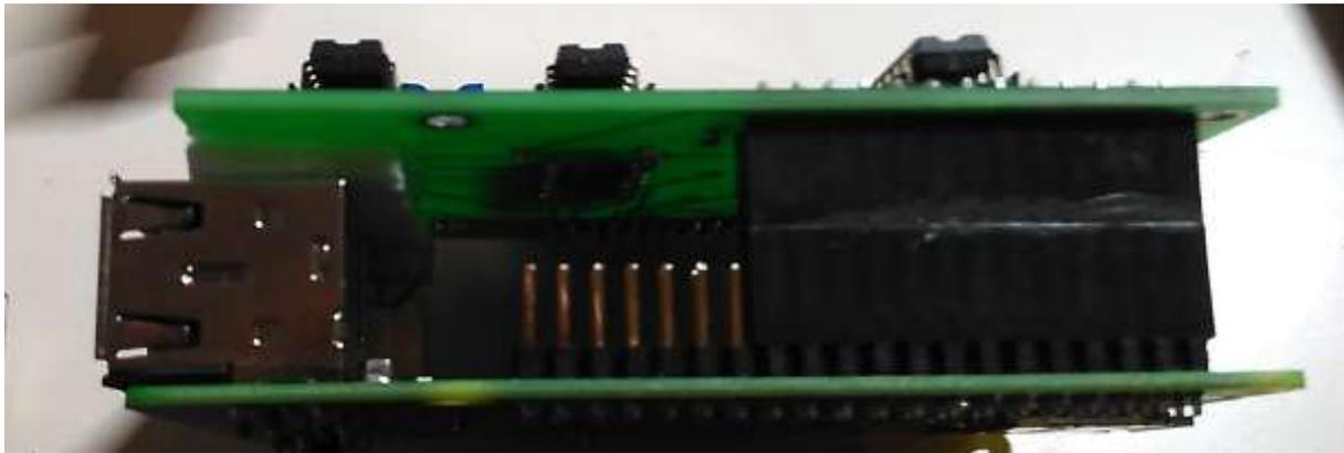
You should then secure the Retro-Printer module to the Single Board Computer by using the supplied spacers and bolts.
